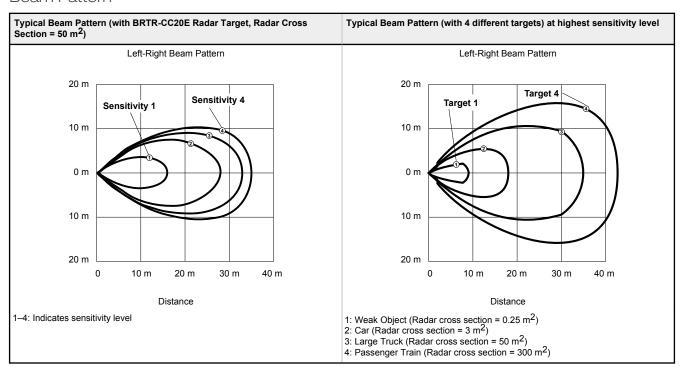
**Note:** The effective beam pattern depends on the sensitivity level and target properties.
